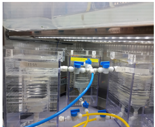
Fig. 14. Parallel connection of three separation apparatuses.
