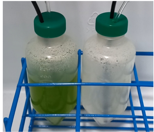
Fig. 13. Homogenization of chlorella and YCT using aeration.
